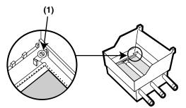
Lift and twist the burner assembly slightly, to separate the crossover tube(1) from the burners. Remove the burners from the cooking box.
